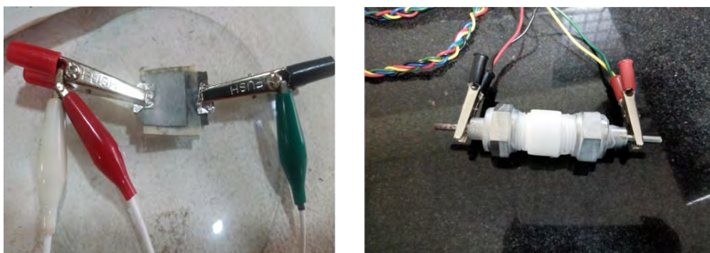
Fig. 4.19 Photographs of prepared electrodes connected to CH instrument
