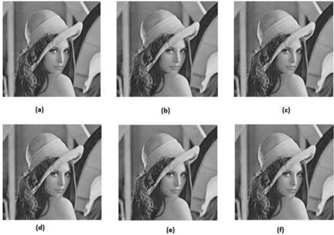
Figure 4.3 (a)Original lena image(512X512) compressed by using proposed method at (b)20% with PSNR 36.23db;(c)40% with PSNR 35.29db;(d)60% with PSNR 35.08db;(e)80% with PSNR 33.29db;(f)85% with PSNR32.33db;
