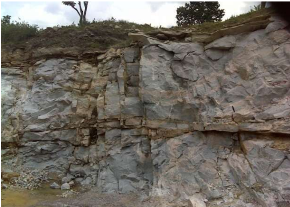
Fig. 3.19. Three sets of joints (mural) in leucocratic gneiss observed at Banavara quarry
