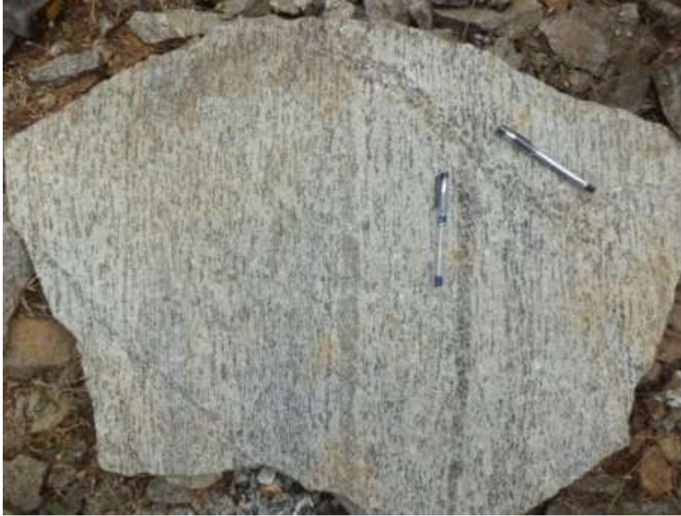
Fig. 3.3. Leucocratic gneiss with typical foliation can see and the sample was collected at Jakkanhalli quarry
