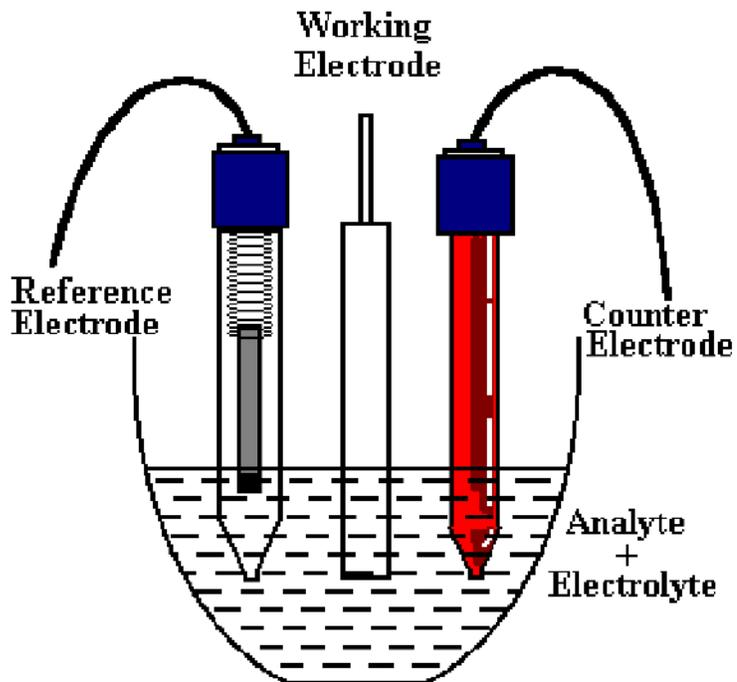
**Fig. 2.3.** Schematic representation of an assembled electrochemical cell containing an electrolyte solution, sparging device, and the three electrodes (WE, RE, and CE) for cyclic voltammetric experiments
