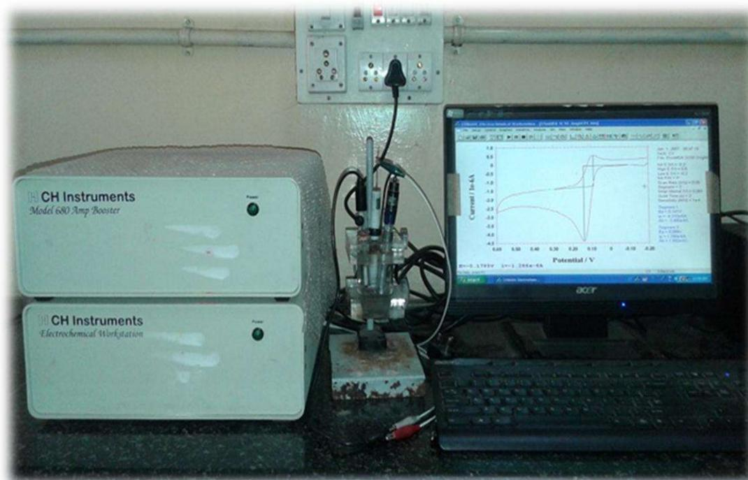
**Fig. 2.2.** Experimental set set-up used to record all electrochemical measurements
