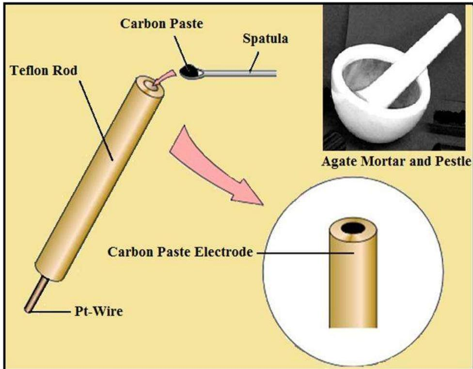
**Fig. 2.4.** Carbon Paste electrode, Preparation and Filling
