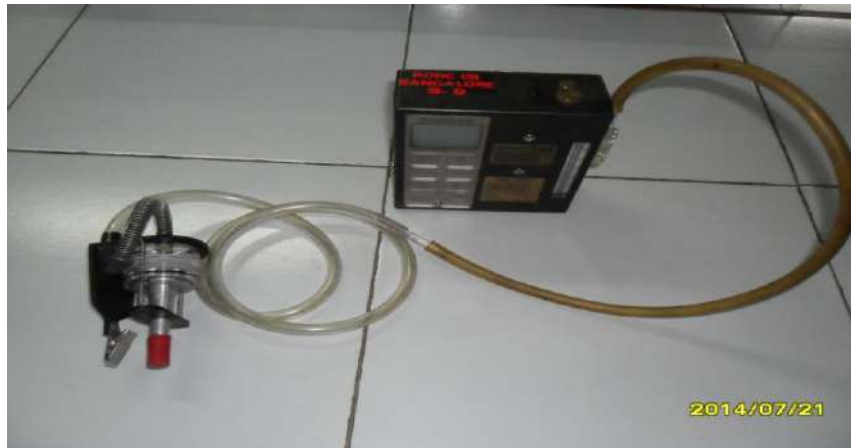
Figure-3.9: Personal Sampler with PTFE filter paper and sorbent tube for PAHs Sampling
