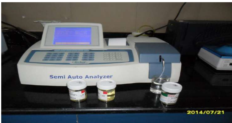
Figure -3.19: Semi Auto Analyzer for urinary creatinine estimation
