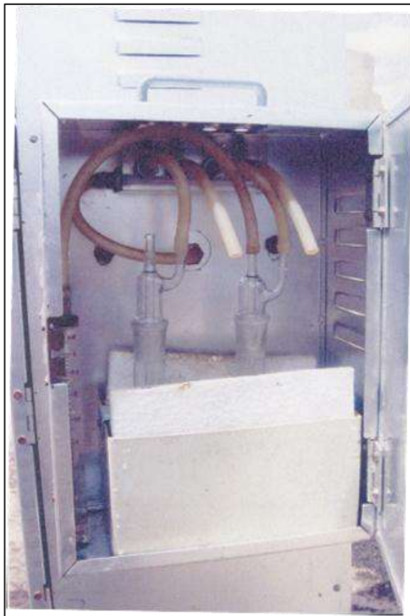
Plate 3.3 View of Gas Collection Arrangement on High Volume Air Sampler
