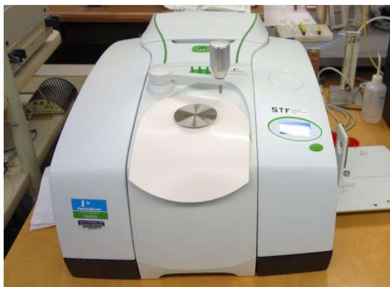
**Fig. 2.4 Fourier Transform infra-red (FTIR)spectroscopy**
