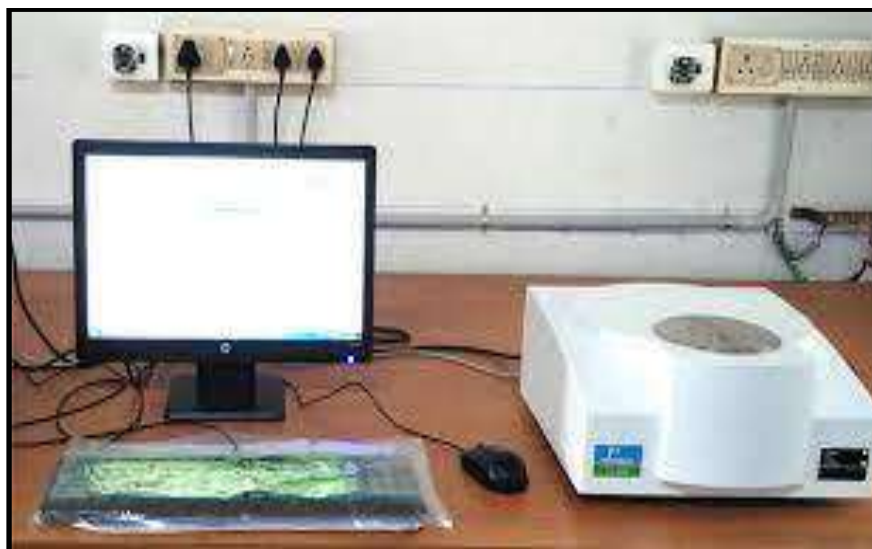
Figure 2.5. TGA/DTA analyzer (Make: Perkin Elmer, Country: America).
