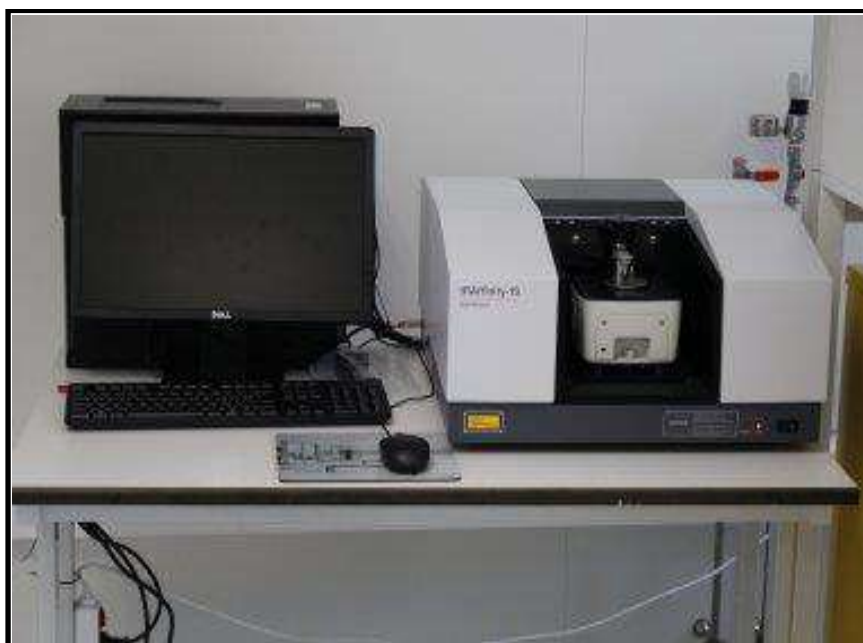
Figure 2.1. The FTIR spectrometer (Make: Shimadzu, Country: Japan).
