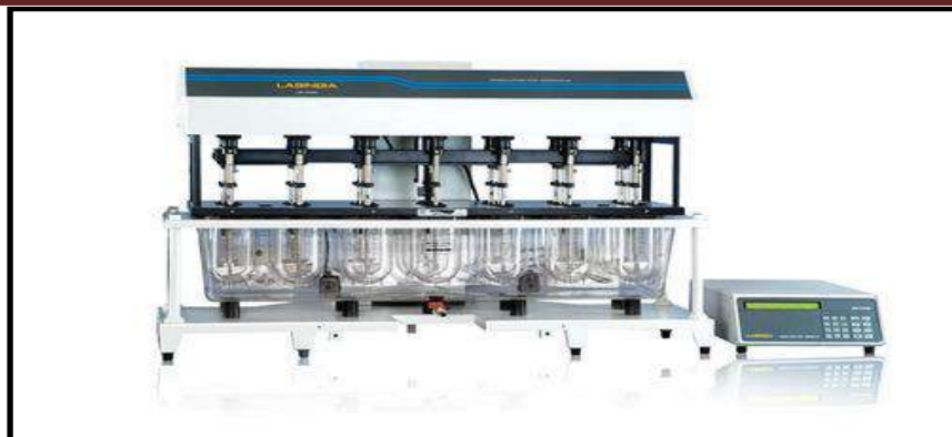
Figure 2.7. Dissolution apparatus (Make: Labindia, Country: India).
