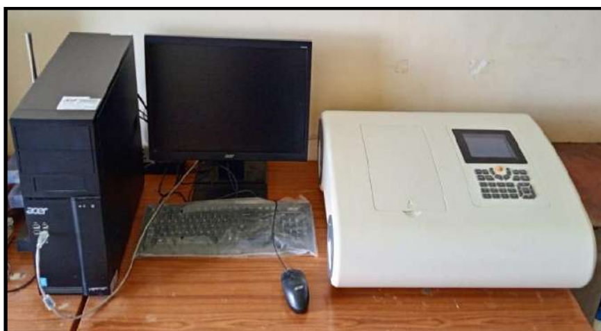
Figure 2.8. UV-Visible Spectrophotometer (Make: Metash, Country: China).
