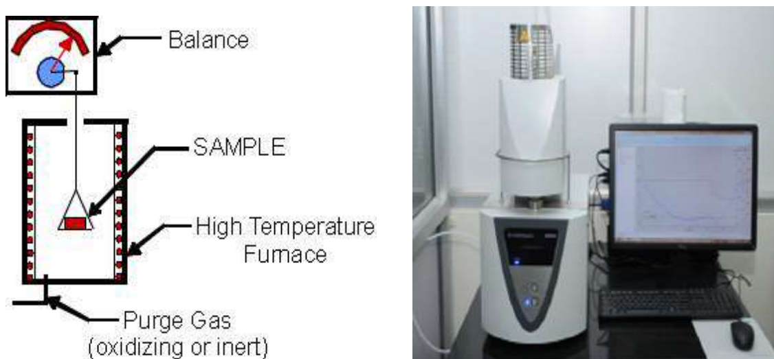
Fig 2.11 Schematic representation and photograph of the TGA measurement
