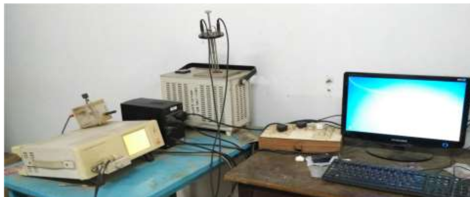
Fig 2.9. Photograph of LCR set up for impedance measurement.
